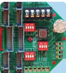
**En** Mother Board: Wiring board; every Rx/Tx in the tower as well as all the peripherals (heater, tamper, accessories) wiring become fixed in this board. To avoid condensation, it includes a thermostat that activates the heaters and the fan, if so configured, in case of low temperatures. Includes alarm output, antisabotage tamper and anti climb tamper outputs and photoelectric beams environmental disqualification output.
