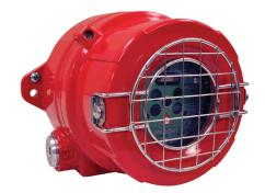
Conventional and older technology UV/IR detectors, using narrow band 4.3 micron IR sensors, will not always respond to smoky fires or if the detector lens is contaminated with oil and other substances since both UV and 4.3 micron signals are attenuated, obscured or absorbed by thick smoke or detector lens contaminations. All UV sensors will be attenuated to some degree.
