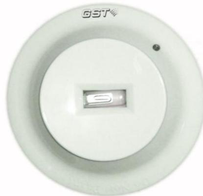
A fixed installation direction is ensured by the location elements on the detector and the base. Fix the base with two tapping screws, and then align mark C on the detector with A on the base, rotate the detector to align mark C with mark B (Refer to Fig. 1 and 2 for the position of the marks), the detector will be fitted to the base.
